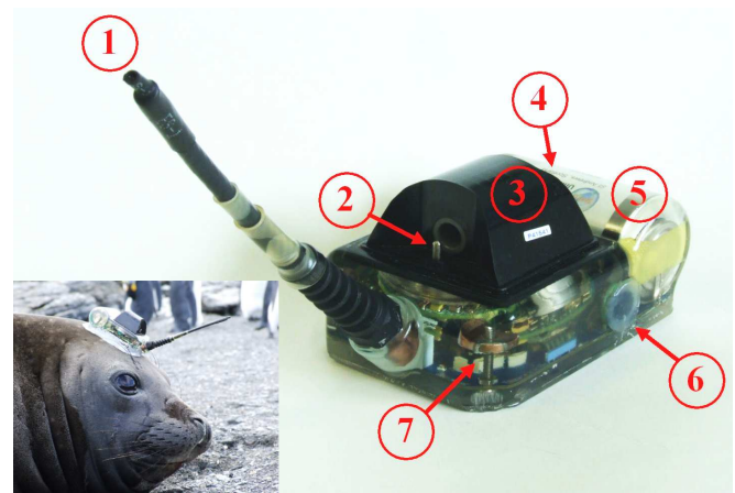
Fig. 1. Picture of a CTD-Satellite Relay Data Logger (CTD-SRDL) with antenna (1), temperature probe (2), inductive cell (3), pressure sensor (not visible) (4), battery (5), communications port (6) and wet-dry sensor (7). Insert: CTD-SRDL deployed on a southern elephant seal.
